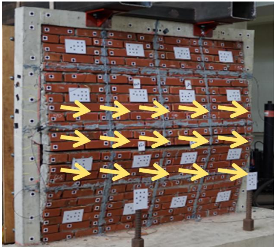
Figure 8. Loading direction (The yellow arrows indicate loading direction).
