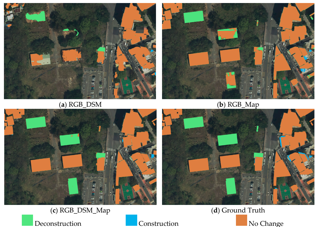
Figure 9. Close look of Figure 7 left “Deconstruction” area: (a) results of RGB_DSM; (b) results of RGB_Map; (c) results of RGB_DSM_Map; and (d) ground truth.
