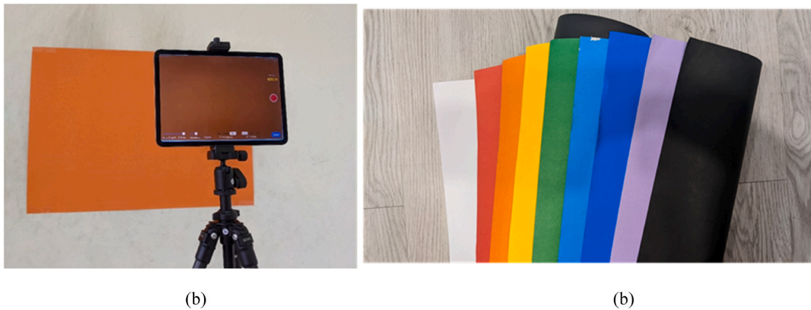
Fig. 4. Configuration of the target's color analysis: (a) setup of the instrument; (b) nine colors used in this experiment. (For interpretation of the references to color in this figure legend, the reader is referred to the Web version of this article.)
